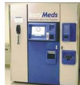
David Samson / The Forum The InstyMeds machine at Innovis Health in Fargo dispenses prescription medicine much like a vending machine.
